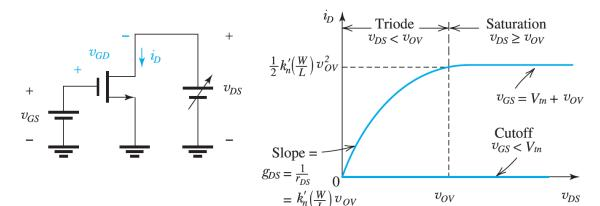
$<sup>{}^{0}</sup>$ In the triode,  $i_{D}$  is controlled by three terminals (hence the name triode), unlike in the saturation mode, where the transistor's operation is controlled by two terminals
